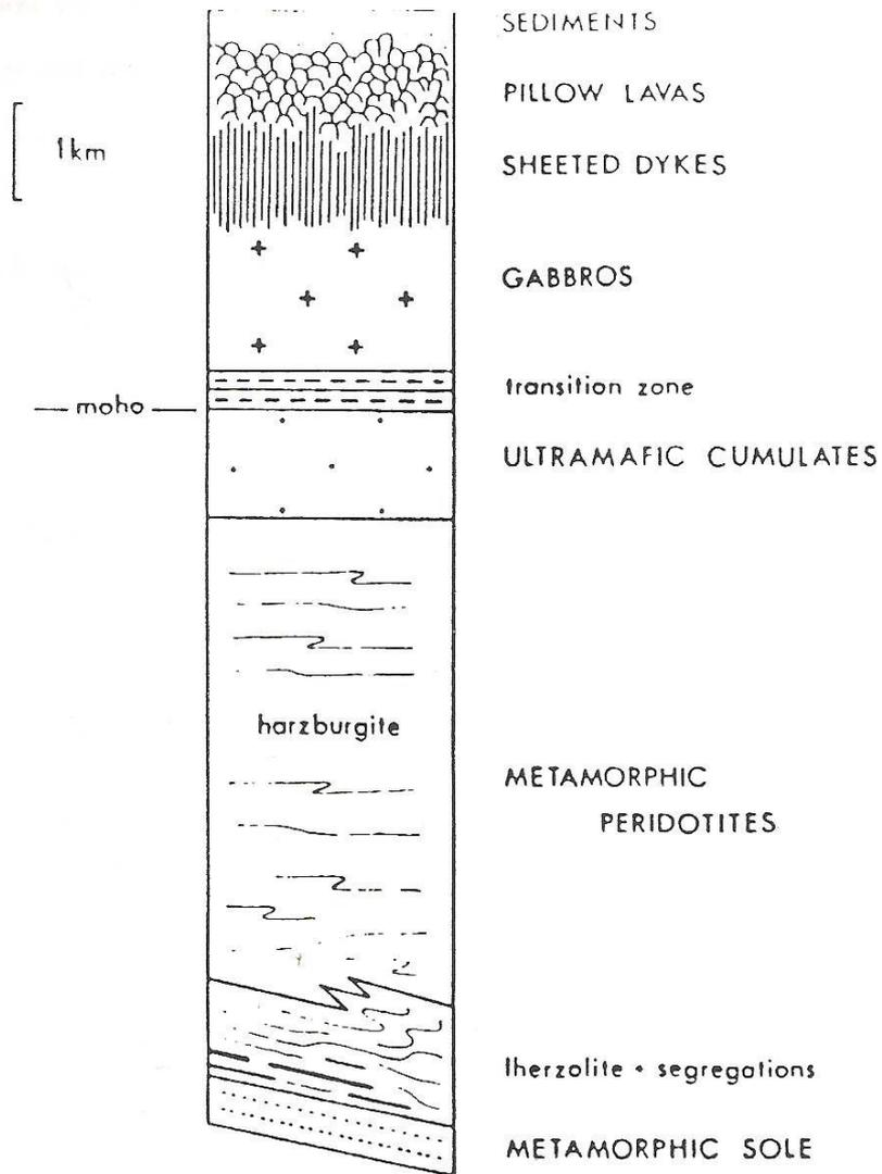
Simplified and idealized cross-section of an ophiolite showing internal components, including positions of lherzolites and mafic segregations in the mantle sequence (metamorphic peridotites) and metamorphic sole.
